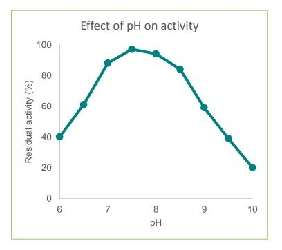
Figure 1. Effect of pH on thermolysin activity (0.5% casein, 35°C, 10 min incubation)
